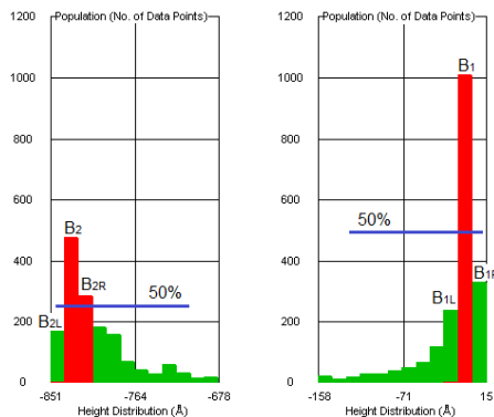
Figure 8. The left and right histograms (zoomed in from Figure 7) show the application of B_{\%} criteria to determine the modes. M_1 = top surface of the dishing structure, with the data from B_1 only. M_2 = bottom surface of the dishing structure, with the data from B_2 and B_{2R} . Since M_1 - M_2 are separated by > 500 \text{ \AA} , M_D criteria, M_2 is a valid mode.
