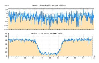
Figure 4. (TOP) Comparison of noise floor profile with Peak-to-Valley value of 27nm and (bottom) shallow SIMS crater with depth measured at 72nm.
