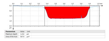
Figure 9. Volumetric analysis using Apex software.
