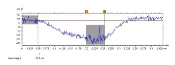
Figure 8. Shallow SIMS crater with 23nm depth measurement.
