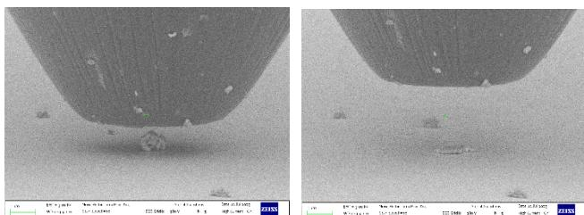
Figure 5. InSEM video image of particle compression prior to (left) and following (right) particle crush measurement.
