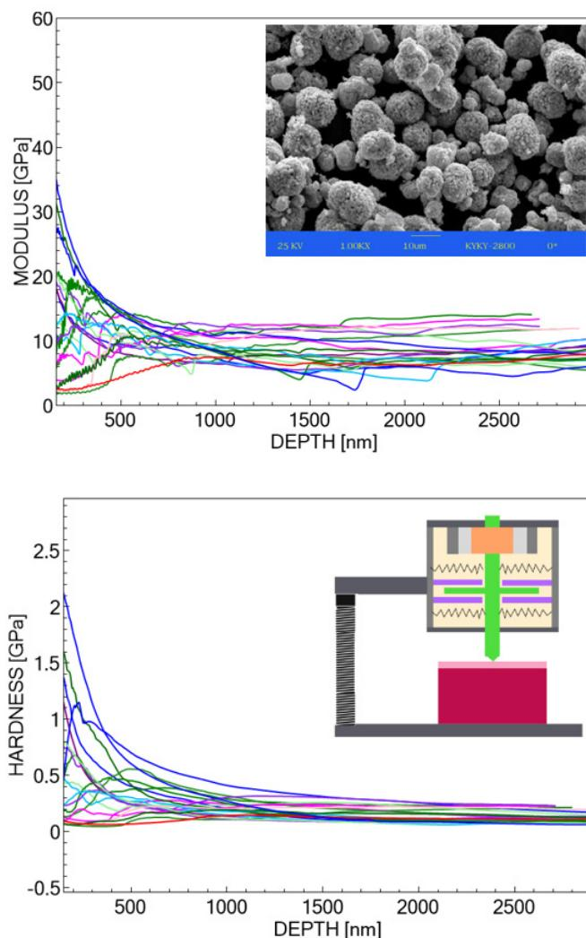
**Figure 2.** Cathode material modulus (top) and hardness (bottom) as a function of indentation penetration depth, with a SEM image of the LiNiCoMnO<sub>2</sub> surface and the KLA actuator schematic. SEM image credit: MTI Corporation.
