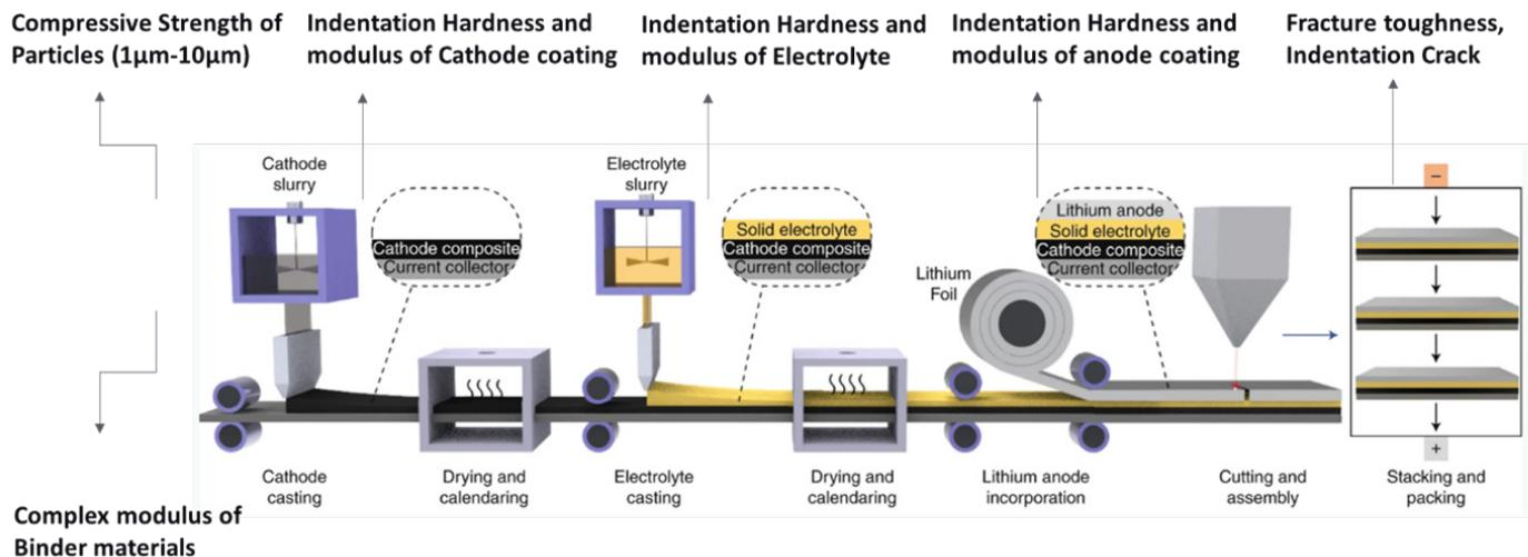
**Figure 1. Schematic of large-scale manufacturing of all-solid-state-batteries (ASSBs).** Polymer and solid electrolyte composites allow for good mechanical processability as well as decreased separator thickness layers to increase cell-level energy density. *Image credit: Tan et al. [2]*
