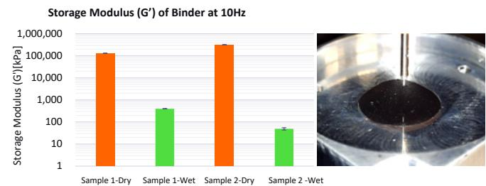
Figure 7. Storage modulus of the binder under dry and wet conditions (left). Nanoindentation measurement in electrolyte solution (right). *Image credit: Toyo Corporation.*
