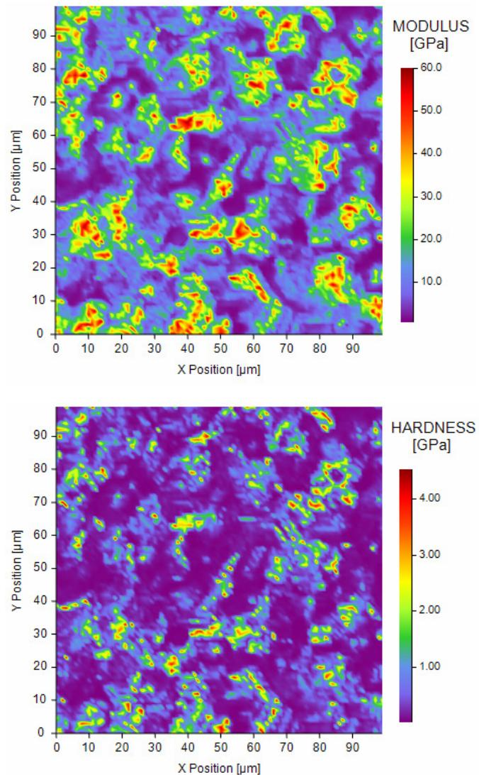
**Figure 3.** Nanoindentation mapping of elastic modulus (top) and hardness (bottom) on a cathode coating.
