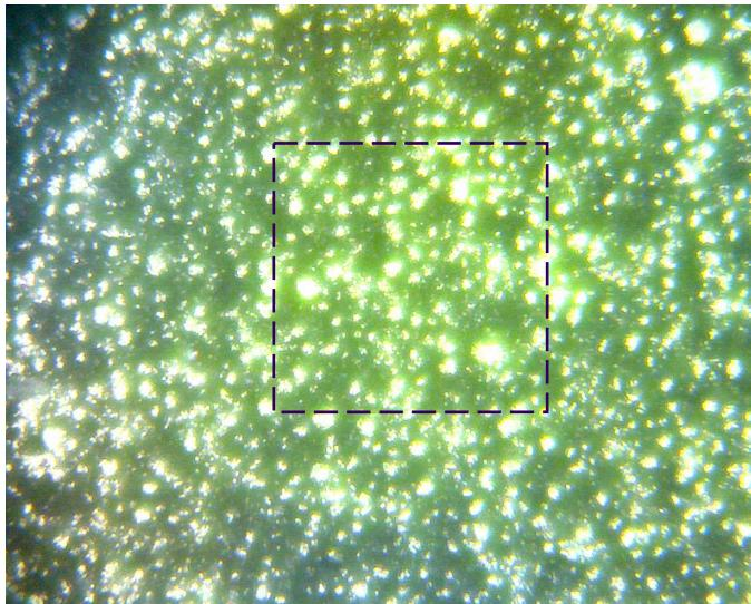
Figure 4. The NanoBlitz 3D test area is shown on the cathode surface.
