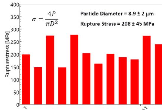
Figure 6. Load-compression response for in situ particle compression (top) and measurements of rupture stress (bottom).
