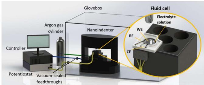
**Figure 8. Example of a glove box environment for the Nano Indenter® G200 system, used to measure load response under argon and fluid environments. Image credit: Scalco de Vansconcelos et al.[3].**
