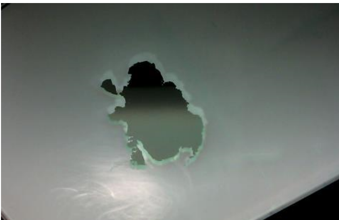
Figure 4. A close-up view of the video image from the F10-RT-UVX shows the removed area of the scattering layer.
